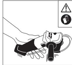
Risk of high vibrations. Wear anti-vibration gloves. Take regular breaks while working.
