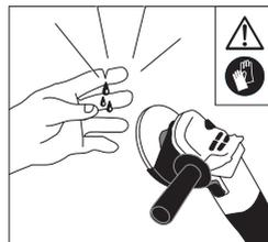
Risk of cutting and abrasion. Keep safety distance from the working area, the abrasive elements, and do not touch any of the moving parts. Always wear protective gloves.
