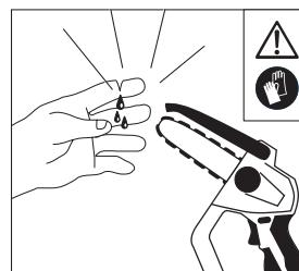
Sharp parts that cause injury. Wear protective gloves and keep a safe distance from the cutting area and the bar.
