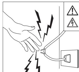
Risk of electric shock with danger to life. Do not touch live parts and keep a safe distance. Before any maintenance, disconnect the plug from the power socket.
