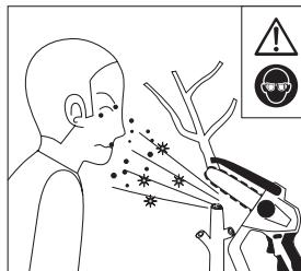
Throwing of material towards the eyes and body of the operator. Wear protective goggles.
